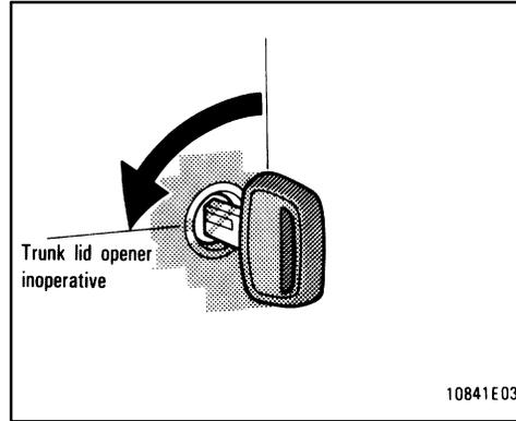
This system deactivates the lock release lever so that things locked in the trunk can be protected.
