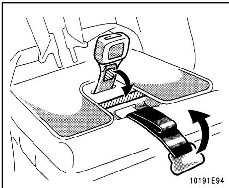
9. To store the built-in child restraint, fasten the shoulder belt clip and return the seat belt buckle using the fastener tapes. Fold up the seat belt adjustment strap (gray tab) in the seat so that the edge of the strap does not come out of the raised seat cushion. Raise the seat cushion and return the head pad by engaging the fastener tapes while pressing the child restraint cushion and head pad firmly.
