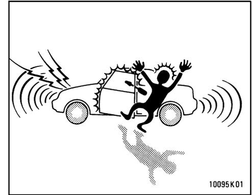
To deter the vehicle theft, the system is designed to give an alarm and keep the engine from being started if any of the side doors, trunk lid or hood is forcibly unlocked or the battery terminal is disconnected and then reconnected when the vehicle is locked.
