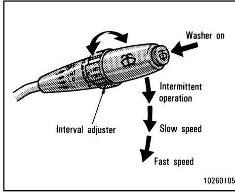
To turn the wipers on, move the lever. To make the washer squirt, push the button on the end of the lever.
