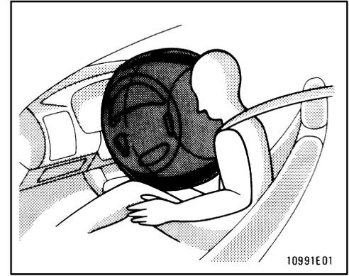
**The SRS (Supplemental Restraint System) airbag is designed to provide further protection to the driver when added to the primary protection provided by the seat belt.**
