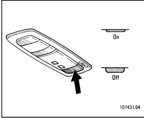
To turn on the personal light, push the switch. To turn it off, push the switch once again.
