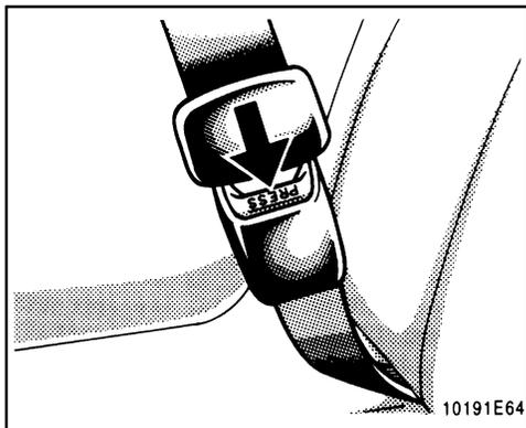
3. To remove the convertible seat, press the buckle-release button.
