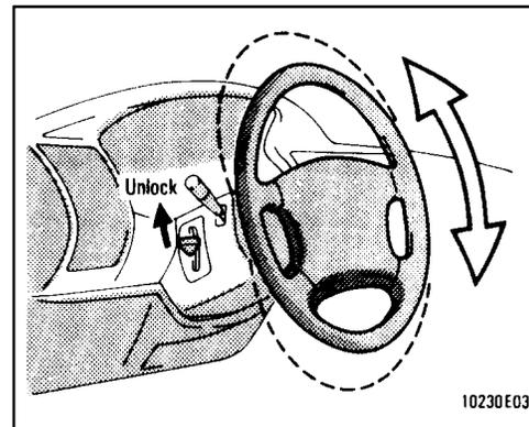
**To change the steering wheel angle, pull up the lock release lever, tilt the steering wheel to the desired angle and release the lever.**
