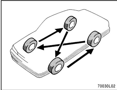
To equalize tire wear and help extend tire life, Toyota recommends that you rotate your tires every 12000 km (7500 miles). However, the most appropriate timing for tire rotation may vary according to your driving habits and road surface conditions.
