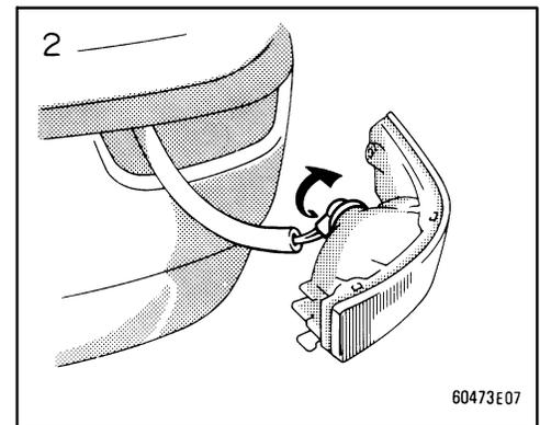
—Rear turn signal, stop and tail, rear side marker, and back-up lights
