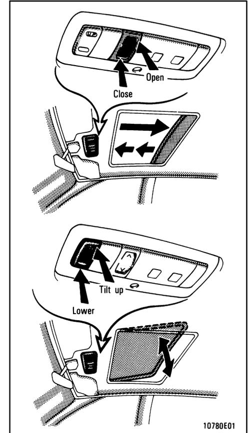
To open the sun roof, push the switch on the “SLIDE” side. Pushing on the opposite side will close it. To tilt up the rear end of the sun roof, push the switch on the “UP” side. Pushing on the opposite side will lower it.
