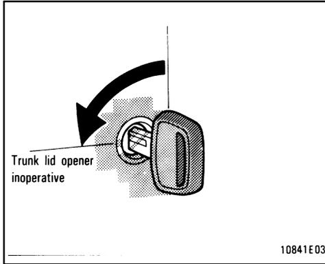
2. After closing the trunk lid, insert the master key and turn it counter-clockwise to deactivate the lock release lever.
