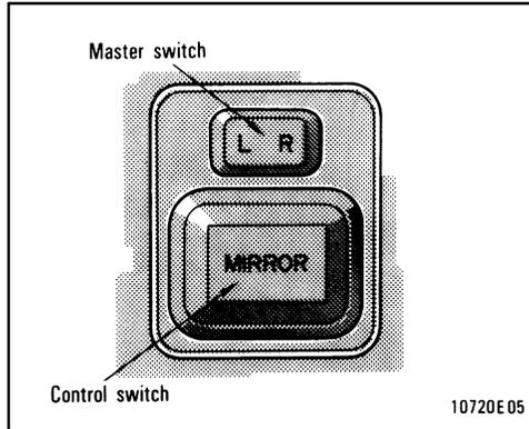
To adjust a power rear view mirror, first push the master switch in “L” (left) or “R” (right) depending on which mirror needs adjusting, then push the control switch in desired direction.
