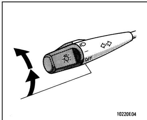
**To turn the lights on, twist the knob on the end of the lever.**
