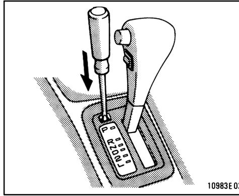
3. Insert the screwdriver or equivalent into the hole to push down the shift lock override button. You can shift out of “P” position only while pushing the button.
