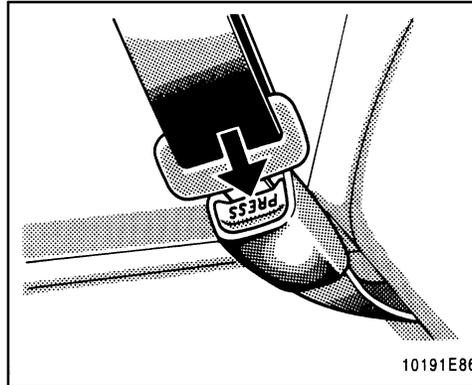
2. To remove the child restraint system, press the buckle-release button and allow the belt to retract.
