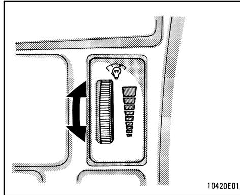
**To adjust the brightness of the instrument panel lights, turn the dial.**
