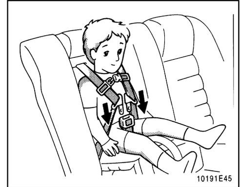
5. Sit the child on the child seat. Place a shoulder belt over each shoulder. Insert the tabs into the buckle.
