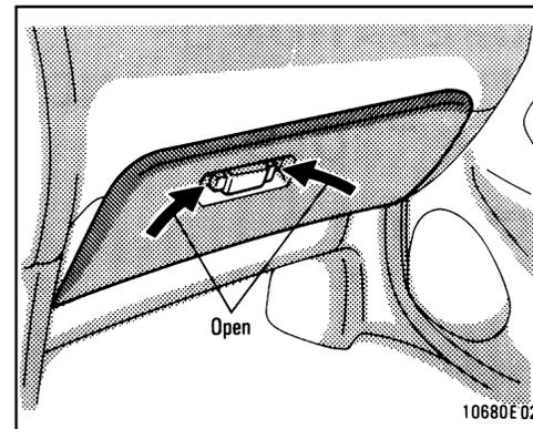
**To open the glovebox door, compress the lock release buttons.**
