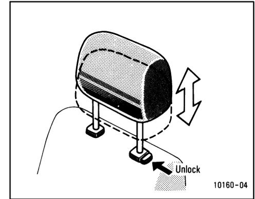
To raise the head restraint, pull it up. To lower it, press the lock release button and push the head restraint down.
