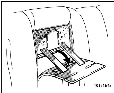
1. **Add slack to the shoulder belts by pulling both of them together while pulling the black seat belt release strap (see step 4 for illustrated instruction). Then pull down the seatback part of the removable pad. Determine the proper shoulder belt slot height for your child. Select the slots at or just above the top of the child's shoulders.**
