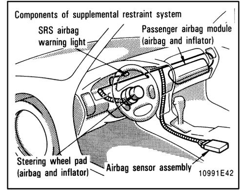
The airbag sensor assembly consists of a safing sensor and airbag sensor.
