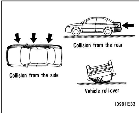
The SRS airbag is not designed to inflate if the vehicle is subjected to a side or rear impact, if it rolls over, or if it is involved in a low-speed frontal collision.
