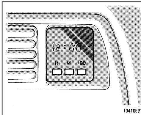
The digital clock indicates the time with the ignition key at the “ACC” or “ON” position. To reset the hour, depress the “H” button. To reset the minutes, depress the “M” button. To adjust the time to full hour, depress the “:00” button.
