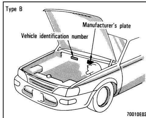
The vehicle identification number (VIN) is the legal identifier for your vehicle. Its location is shown in the illustration.
